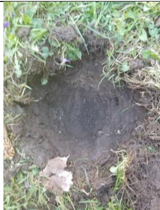
IMAGE 11 TEST PIT SOIL OVERLAYING SUBSOIL
